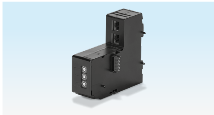
Bus module BCM 500 for connection to the FDU. The address for the fieldbus communication is set using three code switches.
