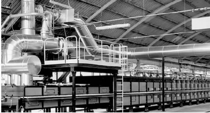
Roller hearth kiln in the ceramics industry
